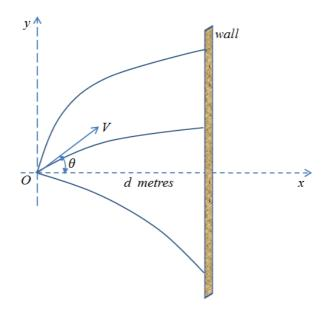
In the diagram above, a large number of projectiles are fired simultaneously from O, each with the same velocity V m/s, but different angles of projection  $\theta$ , at a wall d meters from O. The projectiles are fired so that they all lie in the same vertical plane perpendicular to the wall.
